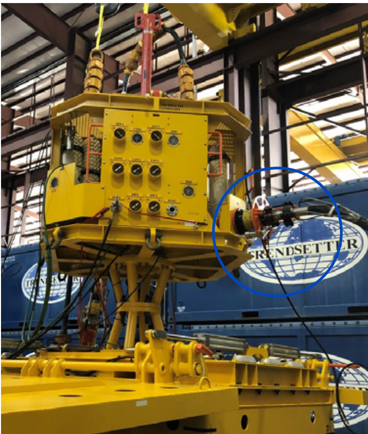
TC2 Hydraulic Connectors Locked by ROV
