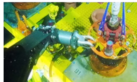
The field-proven TC2 connector features an ROV-friendly user interface for a seamless connection
