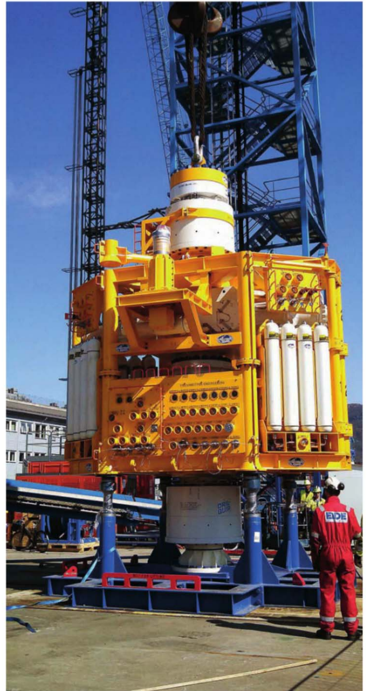
SUBSEA SAFETY: Preparing the mudline closure device for offshore deployment quayside in Norway.
