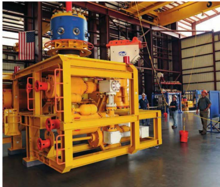
READY TO ROLL: Technicians complete factory testing of the flowpool, which is part of the OSRL containment toolkit.
