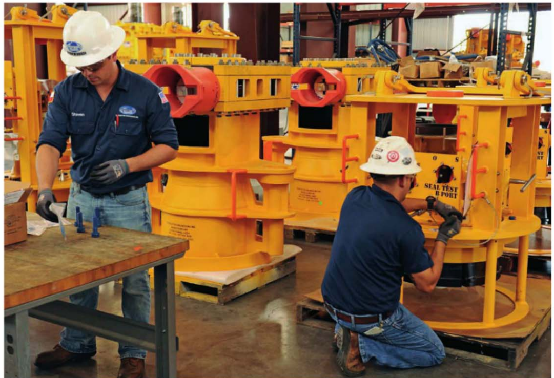
FINAL TOUCH: Engineers assemble the pressure caps and jumper connectors for a Gulf of Mexico project.
